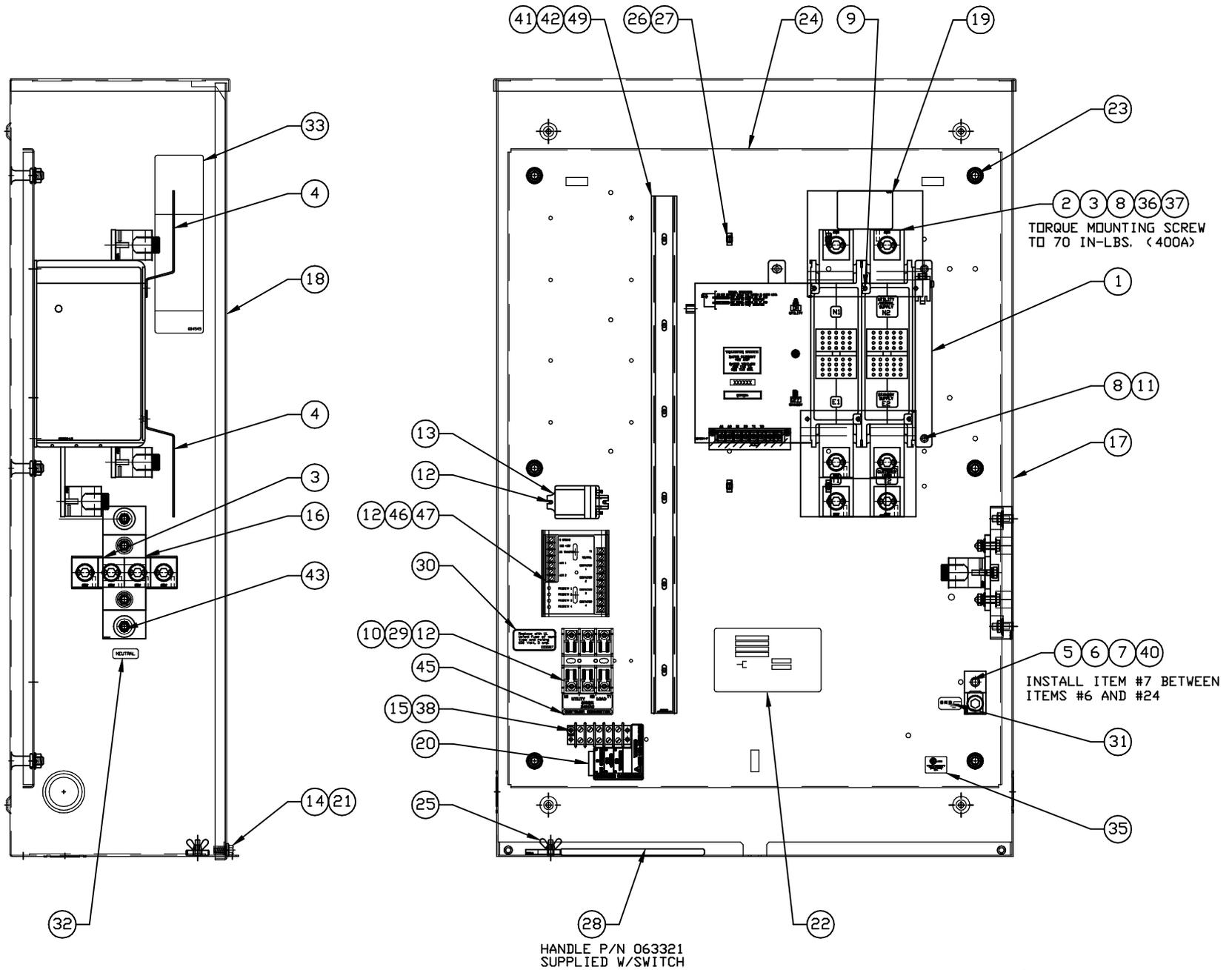
CENTER DECAL APPROXIMATELY 6-1/4" DOWN FROM TOP OF COVER USING ASSEMBLY TEMPLATE
