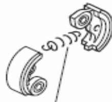
Tension spring 7 (231881-3) Free length: 35 mm
