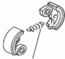
Tension spring 6 (231858-8) Free length: 27 mm
