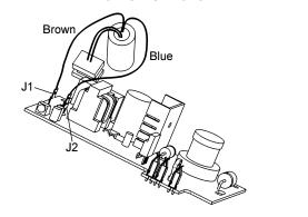
Connect brown conductor of cordset assembly to terminal marked "J1" on circuit board assembly.
