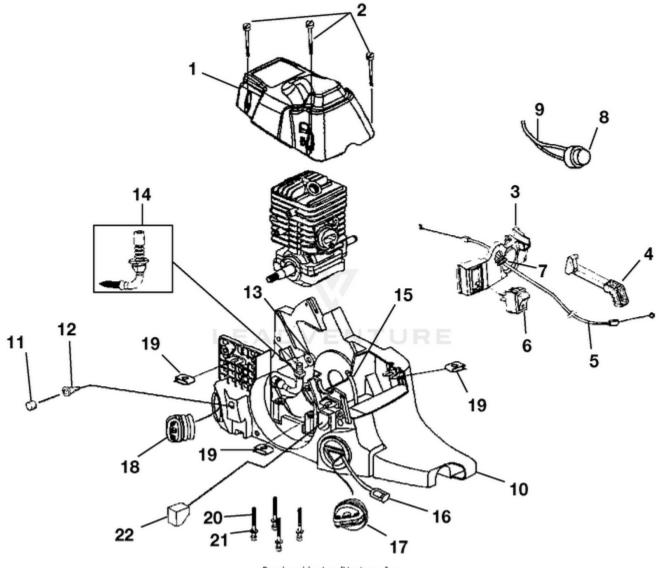
45cc Chain Saw UT-10942 10942-UT 45cc Chain Saw UT-10942 45cc Chain Saw - Engine Housing - Fuel Tank - Oil Tank
