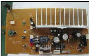
POWER PCB ASSEMBLY No. 22-09-1231 1. PCB with AM antenna (AM antenna not shown in picture)
