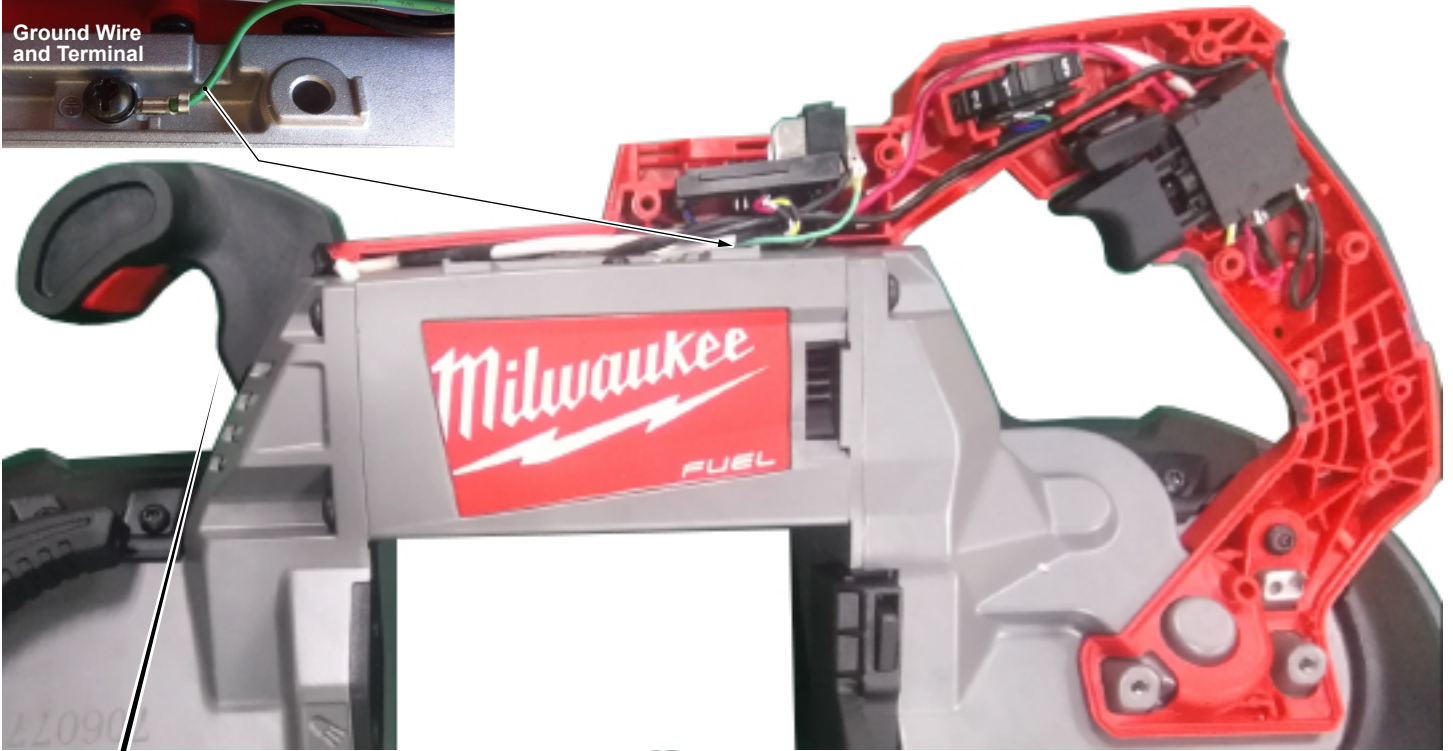
Bottom of T-Handle showing Micro-Switch wire routing
