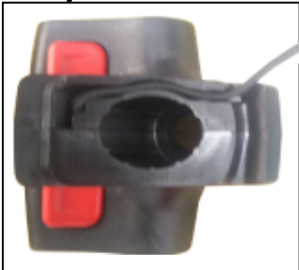
Bottom of T-Handle showing Micro-Switch wire routing
