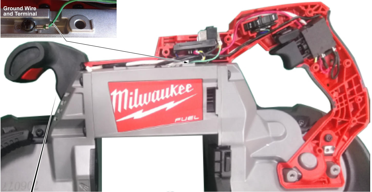
Bottom of T-Handle showing Micro-Switch wire routing
