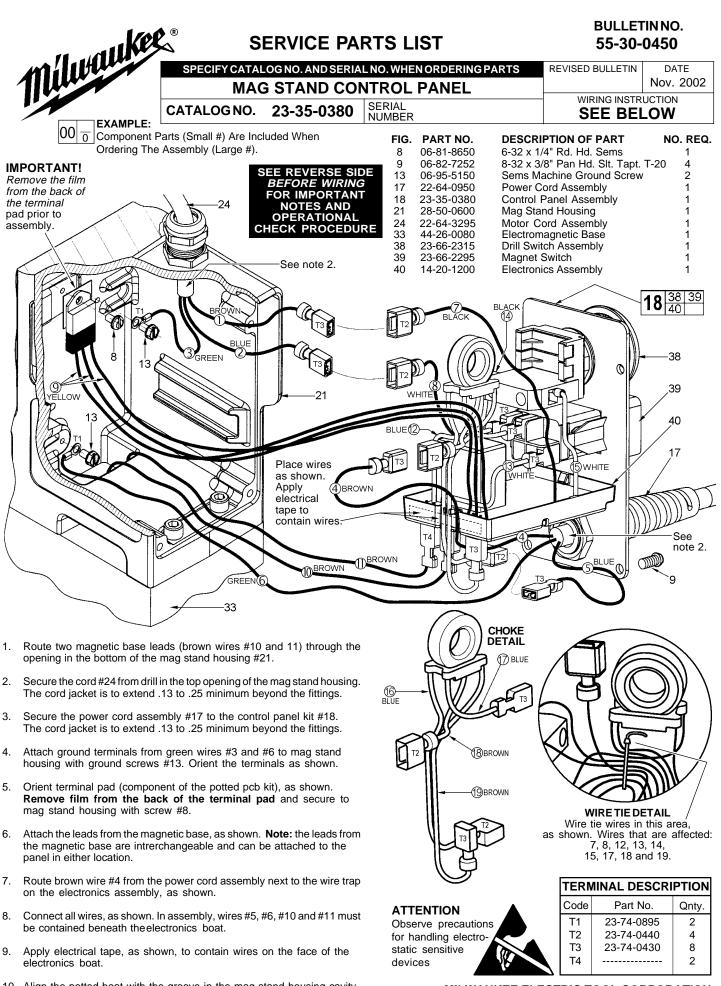
10. Align the potted boat with the groove in the mag stand housing cavity. Gently push the bundle of wires and the control panel assembly into the housing. Avoid pinching wires as the control panel is being installed.
