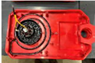
**STEP 1:** Obtain the previously assembled Connector Plate and Motor Assembly
