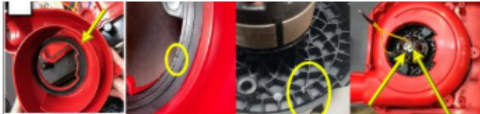
**STEP 2: Obtain (1) Volute, Exhaust and ensure (1) Top, Isolator (31-55-0019) is installed.** Set the volute assembly into place over the motor as shown. Make sure the notch in the isolator matches up correctly with the notch on the motor. The terminal ground wire should be in the 1 o'clock position as shown.
