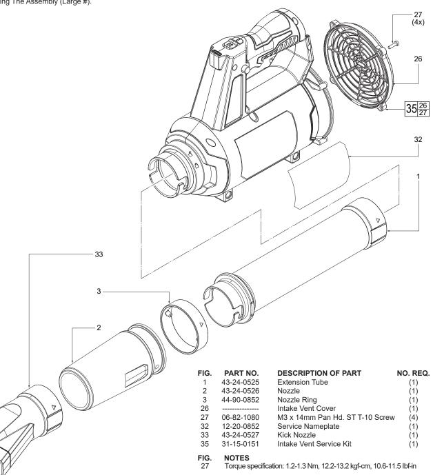
32 A clean, dry surface is essential for proper performance for any adhesive system. The area intended for application of any adhesive label or nameplate must be prepared by cleaning with isopropyl alcohol. The solvent is to be applied with a clean, lint free applicator and the surface allowed to dry before applying any label or nameplate.
